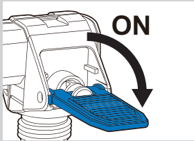
Dials for smooth ON/OFF flow control
